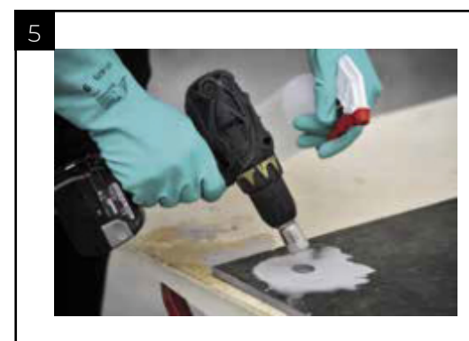
5. Diamond tool for wet drilling
